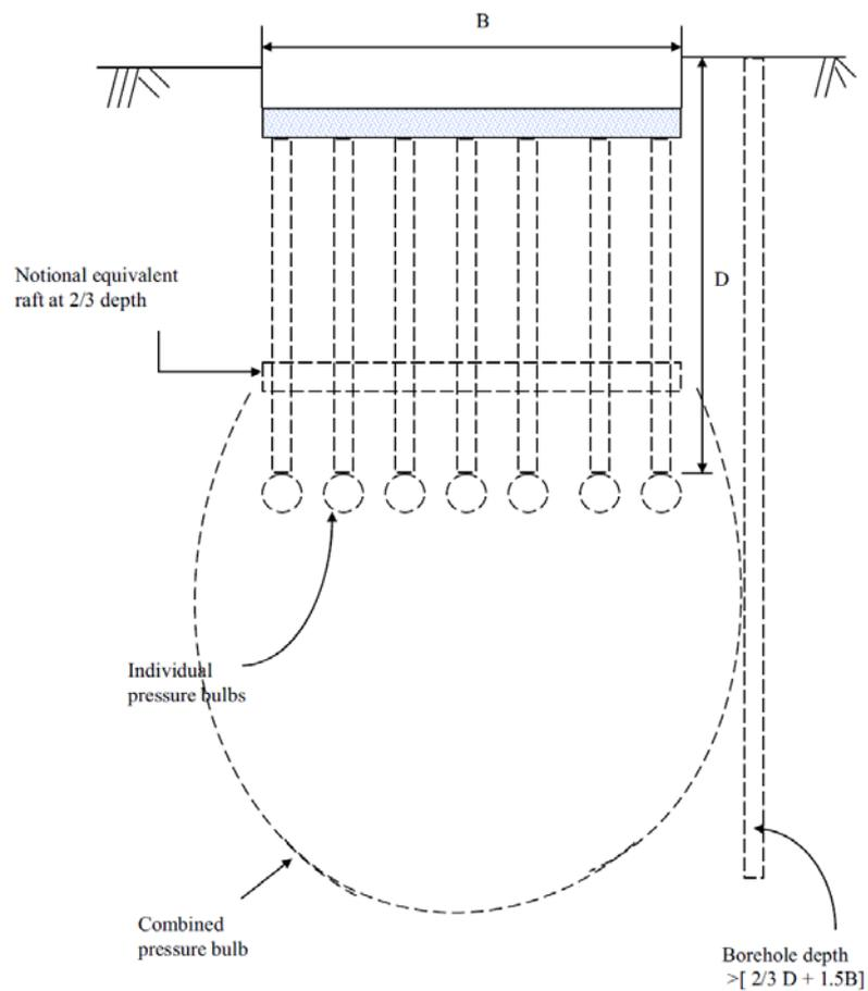
**Figure 3** Estimated borehole depths based on pressure bulb for large structure on friction piles (ref: Clayton *et. al.*,1995).
