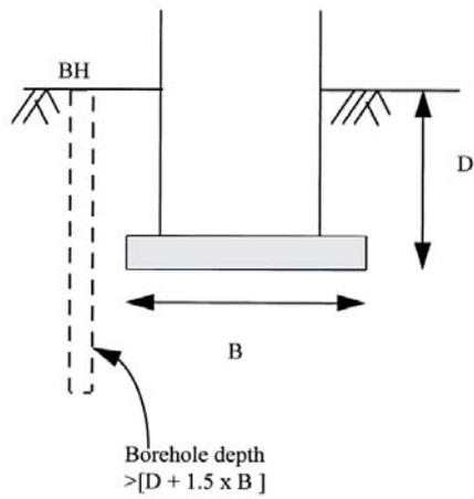
**Figure 2** Estimated borehole depths based on pressure bulb for structure on isolated pad or raft (ref: Clayton *et. al.*,1995).
