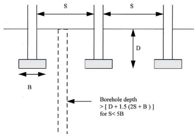
**Figure 1** Estimated borehole depths based on pressure bulb for closely spaced strip on pad footings (ref: Clayton *et. al.*,1995<sup>2</sup>)
